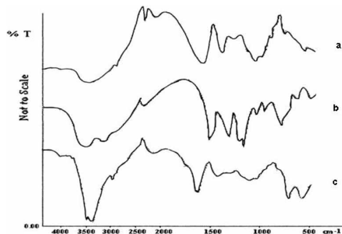
Fig. 4. FTIR spectra of (a) unloaded bead sample, (b) drug, (c) drugloaded bead sample.
